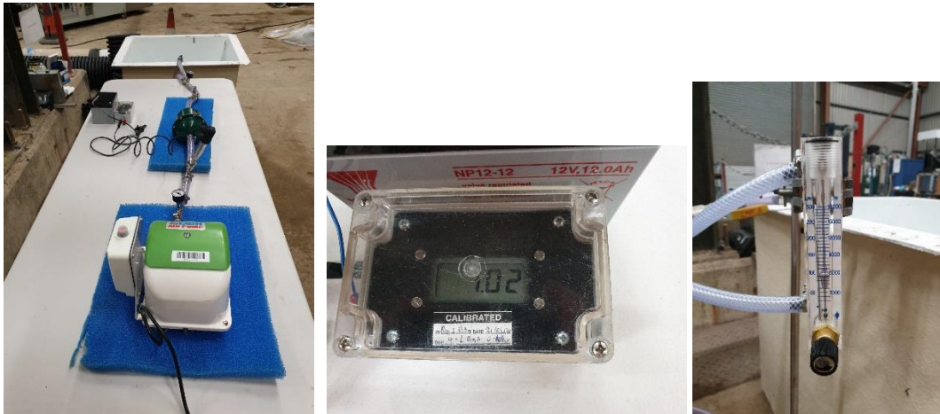
Figure 2 Test set up, pressure measurement readout and air flow measurement.
