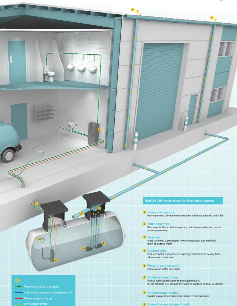
Controls the distribution of rainwater from tank to utilities
